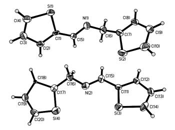
Fig. 1. ORTEP diagrams of compound 1a at the 50% probability level.
